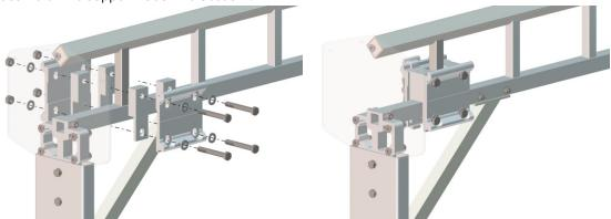
13. Hang the cassettes with the suspension brackets in the mounting plates on the Twins Piazzola<sup>®</sup>. Fasten the socket screws on the bottomside.
