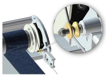
14. Hook the cover support into the bottom cover and place it alongside the socket screw that projects through the cover.
