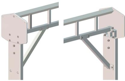
11. Fasten the strut with M8 bolts and check that the structure is level.
