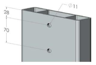
Attention! If water enters in the support, drill a hole in the bottom of it. This to prevent damage from frost.
