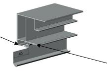
Screw in the corner or – rivet to the side guide.
