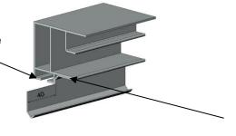
Screw in the corner or – rivet to the side guide.
