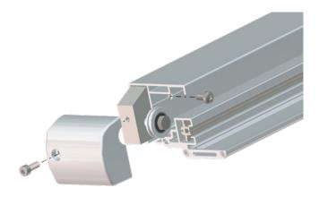
14. Install the central beam for the fabric support between the brackets and fasten them with socket head bolt M8 x 30 mm.
