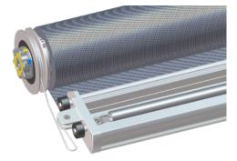
13. Disassemble the top part of the aluminium motor support and the bearing block. Place the complete internal mechanism with front profile into the bottom cover. Fasten the entire core with the top part of the motor bracket and the bearing block.
