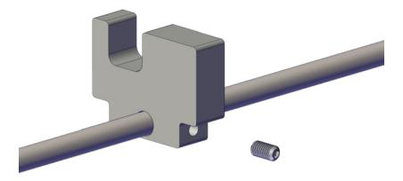
Take the tensioning wire through the tensioning wire mounting blocks and the cover profile. Fasten the tensioning wire mounting blocks in the clamping plate with M8 x 25 mm bolts.
