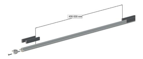
5. Slide the pvc guide, optional central beam supports and top distance brackets in the side guide and fasten them slightly. Install the guide plate at the side with the 2 pre-drilled holes.
