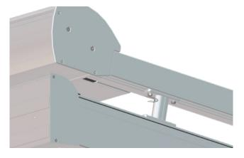
6. Fasten the side guide to the top cover support with cylinder head plate screws M6 x 14 mm.
