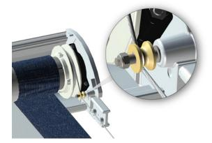
15. Install the top cover and fasten with self-drilling screw 3.5 x 9.5 mm. Click the cover profile on the front profile.
