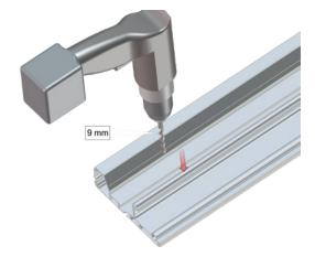
3. Drill holes of 6.5 mm with aid of the drilling template in the slot of the front profile. Keep about 500 mm distance between the holes. Keep a distance of 700 mm in the middle of the front profile.
