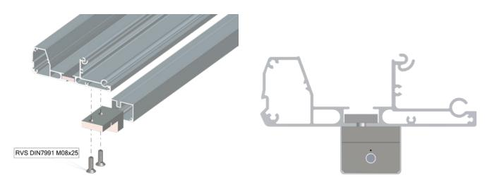
6. Keep at both sides of the mounting block and the cover profile a distance of 2 mm. Fasten the cover profile through the holes of 6.5 mm.
