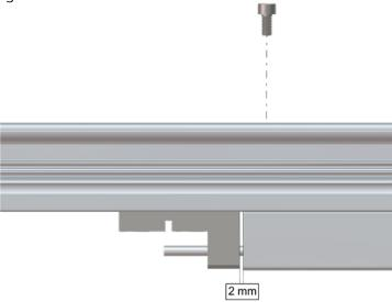
7. Fasten the hexagon connection nut with a washer to the side of the tensioning wire with screw-thread. On the other side the clamping sleeve with wedge set is positioned.
