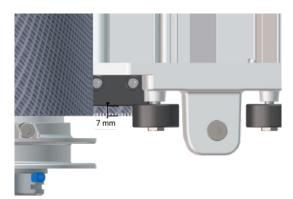
12. Pass the cord through the guide block in the front profile. Allow a loop to extend from the front profile. Neatly roll up the rest of the cord and lay it into the front profile.
