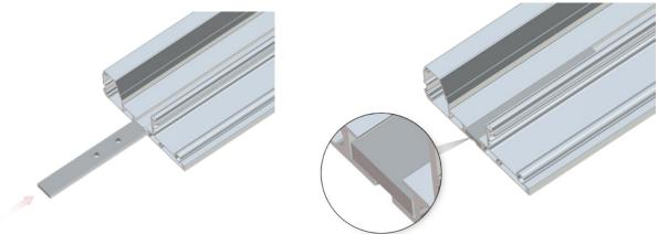
2. Mark the holes and drill hole of 9 mm. Do this on both sides of the front profile. **Note :** Do not drill the holes of the clamping plate !
