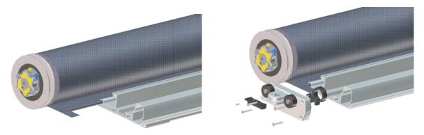
9. Hook the spring onto the eye on the guide block. Slide the support blocks over the springs and fasten with self-drilling screws 4.2 x 13 mm (2 pcs. per spring).
