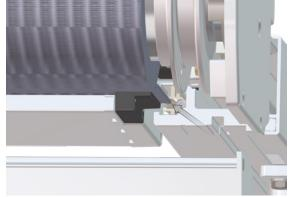
5. Fasten the hexagon bolts of the distance brackets, so the side guides cannot glide.
