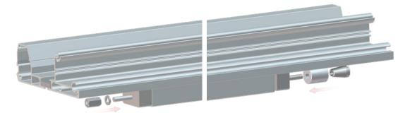
8. Turn the hexagon connection nut tight to tension the front profile straight.
