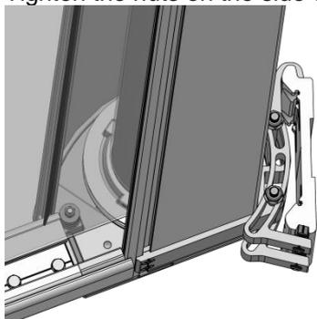
43. Hook the springs on the left and right into the screw eyes of the guide blocks.
